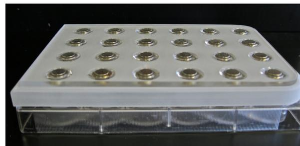
**Figure 1. 24-well Bio-Assembler™ magnetic drive on top of standard 24-well tissue culture plate.**
