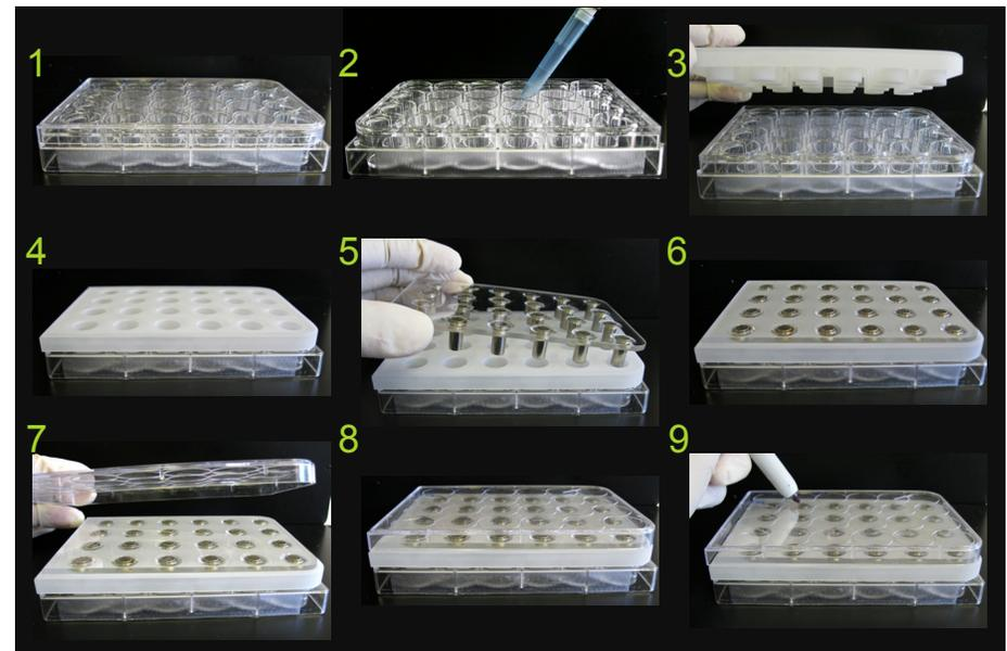
**Figure 4. Steps for assembly of 24-well plate and magnetic drive.**
