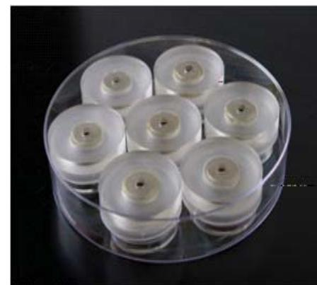
Figure 1. Seven single-well petri dishes with large-magnet Bio-Assembler™ magnetic drives on top.
