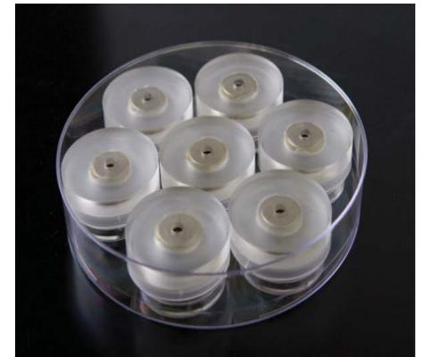
Figure 4. (Left) Assembly of petri dish and magnetic drive. (Right) Petri dishes in petri dish holder. The small-magnet magnetic drive is shown.
